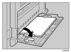
**5** Set the paper size using the printer driver or the control panel.
